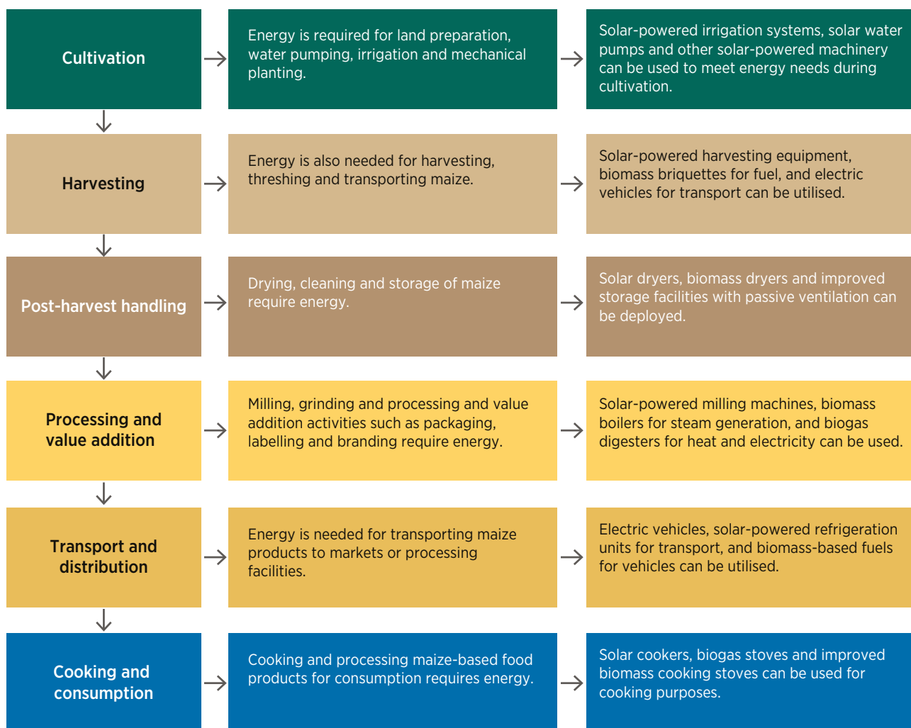
Figure 3 Energy needs at every stage of the maize value chain and the renewable energy solutions
