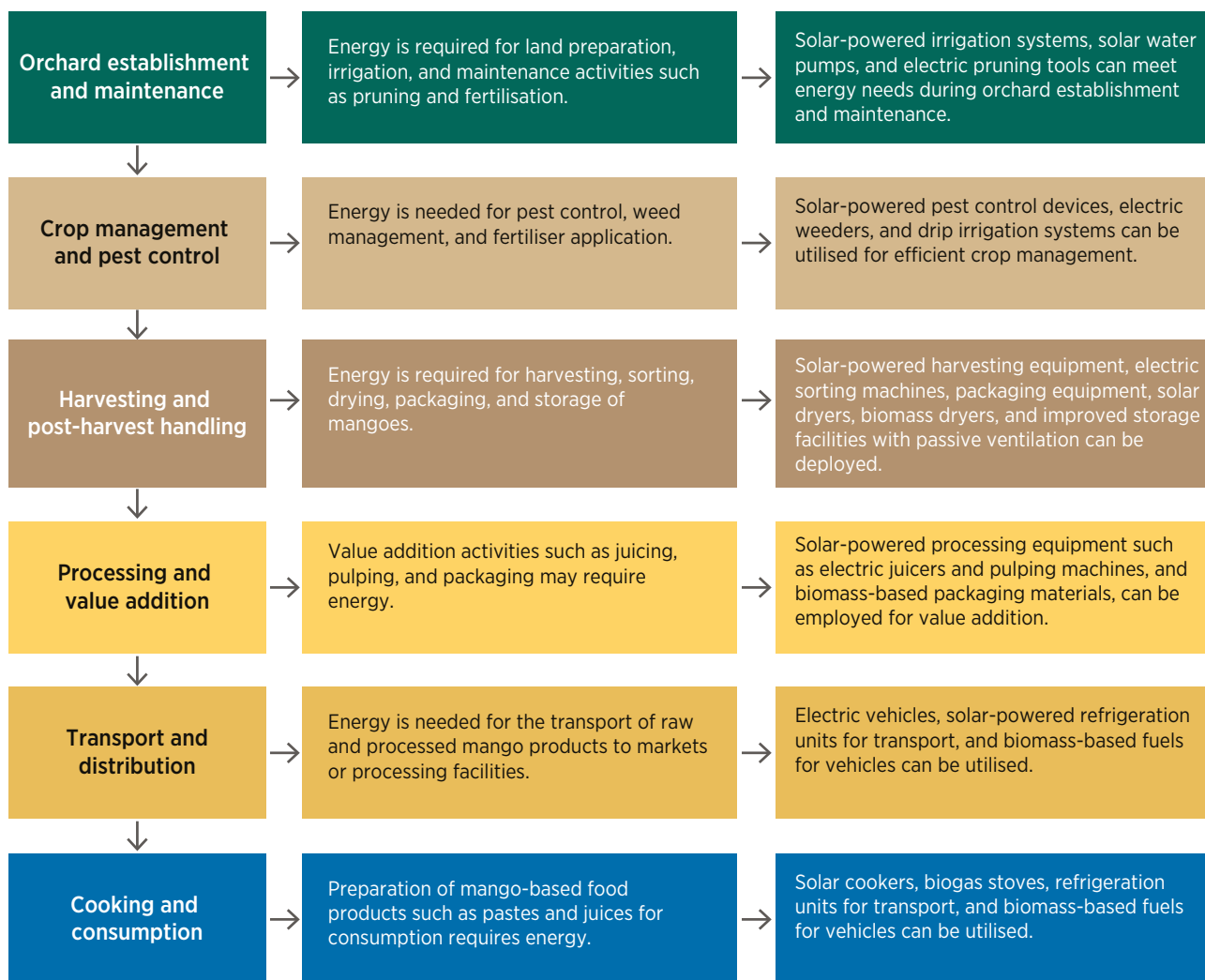
Figure 6 Energy needs at every stage of the mango value chain and the renewable energy solutions
