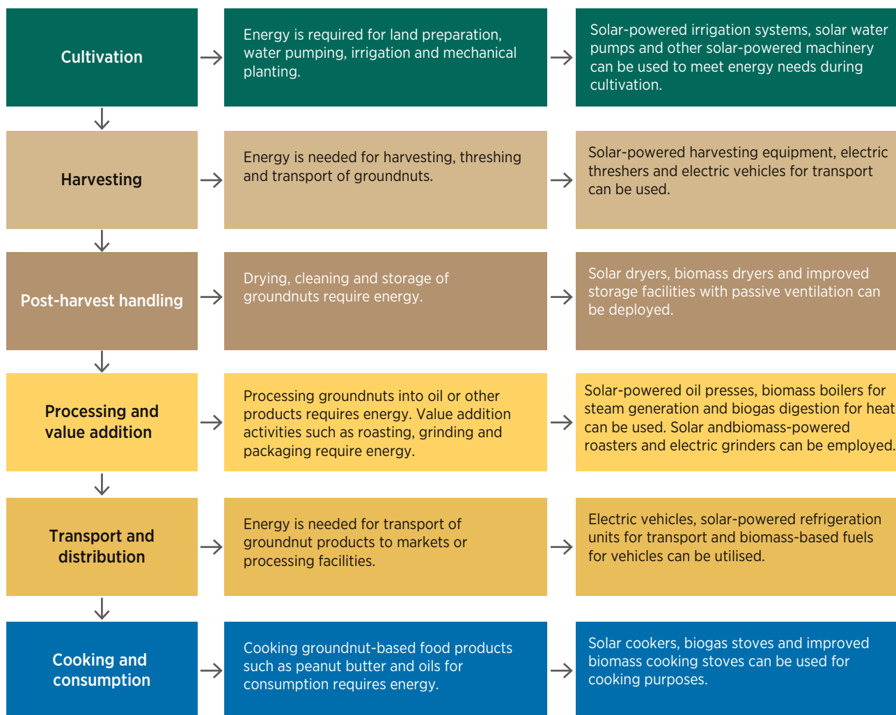
Figure 4 Energy needs at every stage of the groundnut value chain and the renewable energy solutions
