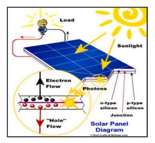
Fig. 5. A picture of the working operation of solar energy.
