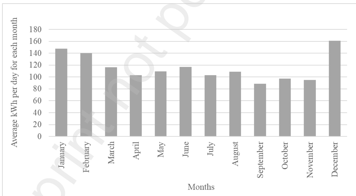
Figure 3: Average kWh per day provided by UB Microgrid for 57 households
